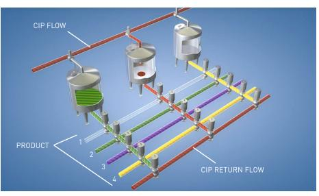
GREEN: TANK IS BEING FILLED YELLOW: TANK IS BEING EMPTIED RED: TANK IS BEING CLEANED
